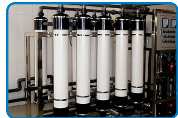
ULTRA FILTRATION PLANT(UF)
